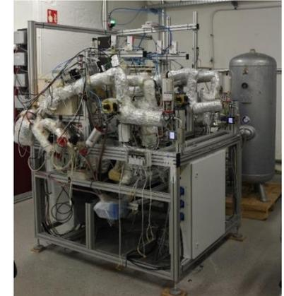
Test rig for small-scale humidifier
