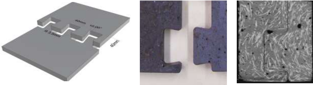
Figure 1: fingerjoints for modular shell structures (left), detail fingerjoint (middle), chaotic fibre distribution, micro CT-scan of the fingerjoint (right).
