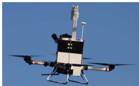
Fig. 9: Quadcopter MesSBAR of the TU Braunschweig for pollutant measurement
