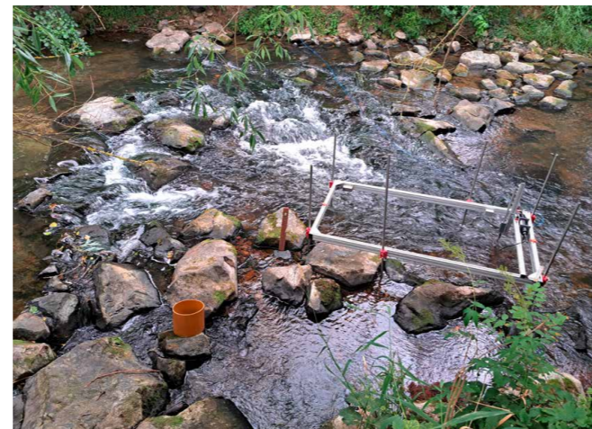
Velocity measurements in the field over an unstructured block ramp (Photo: R. Eikenberg)
