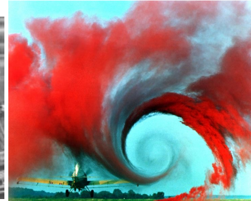
Visualization of tip vortex
